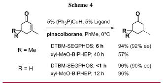
In summary, an especially effective case of ligand-accelerated catalysis has been uncovered for carrying out conjugate reductions of (hindered)  $\beta$ -substituted cyclic enones based on either an in situ-generated SEGPHOS-chelated CuH or a SEGPHOS-modified form of Stryker's reagent. High catalyst turnovers have been realized, very mild conditions prevail, and both yields and enantioselectivities are the highest reported to date for these substrates.
